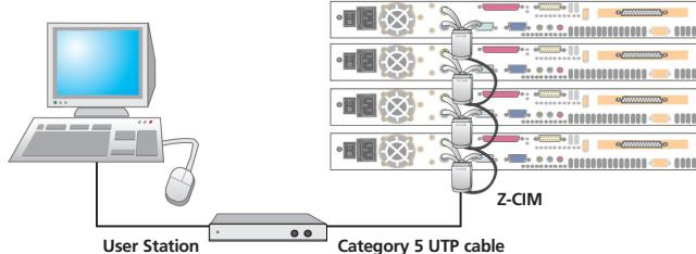
**User Station** – enables a user console (keyboard, video and mouse) to select and control up to 42 servers via a simple, on-screen user interface.
