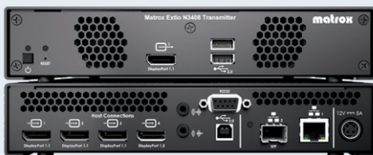
Matrox Extio 3 N3408 Transmitter Appliance (front/back view)
