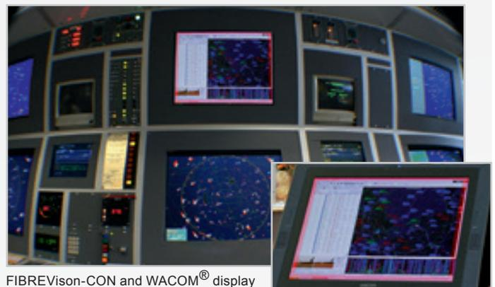
FIBREVison-CON and WACOM® display with active Screen-Freeze function.
