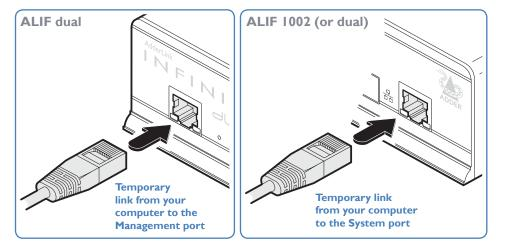
2 Connect the other end of the link cable directly to the network port of your computer.
