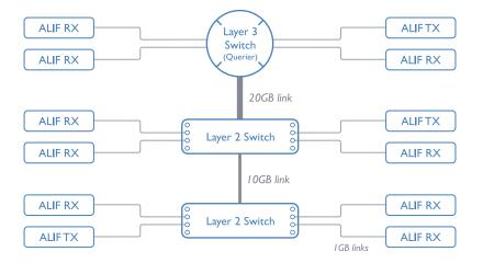
Note: From firmware version 3.1, tree and hierarchical structures of network switches are also supported. The Transmitter now joins its own multicast group so there is always a route from the querier to the transmitter which was previously missing in earlier firmware versions.
