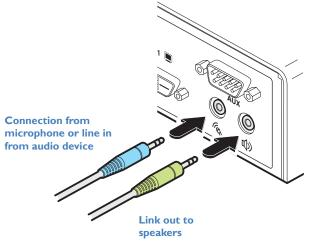
3 Once the unit has been fully connected and powered on, access the RX System Configuration page to check that the *Audio Input Type* setting matches the connection that you have made to the port: *line, mic* or *mic boost* (the latter provides +20dB gain).
