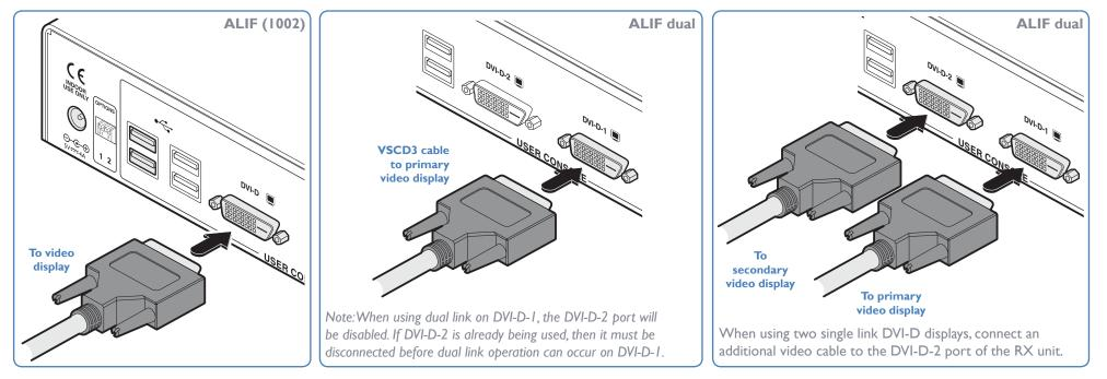
2 (ALIF dual only) If required, connect the lead from the second video display to the DVI-D-2 socket on the RX unit rear panel.
