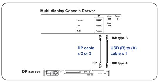
\* DP cable x 2 and USB (B) to (A) cable x 1 for dual display
