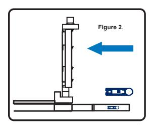
■ Pull and hold both side release buttons when pushing the Multi display console drawer back to the rack. ( shown in **Figure 2** ).
