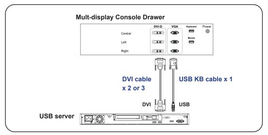
\* DVI cable x 2 and USB KB cable x 1 for dual display
