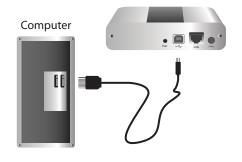
3 Place the Remote Extender where desired. Connect the Cat 5e patch cable from the Link port (RJ45) to a network switch or wall network port connected to a switch and connect the Remote Extender to a power source.
