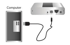
3 Connect the Remote Extender to the AC adapter and a power source.
