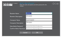
3 Enter the details for this receiver, including the password (required for admin access to the configuration details). Click OK.
