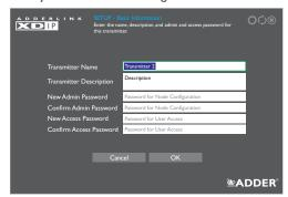
5 Enter the details for this transmitter, including two separate passwords: one for admin configuration purposes and the other to restrict user access to this transmitter. Click OK.
