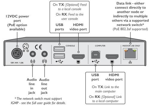
Connect and power on all required nodes. On the console connected to an unconfigured node, that will become a receiver, you should see the Welcome screen. The node's PWR indicator should be red at this stage. If not, restore the node to its default settings (see the rear page). Continued overleaf.
